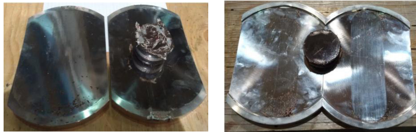
Figure 2: (left) Damage to Bearing set A (right) Damage to bearing set B
