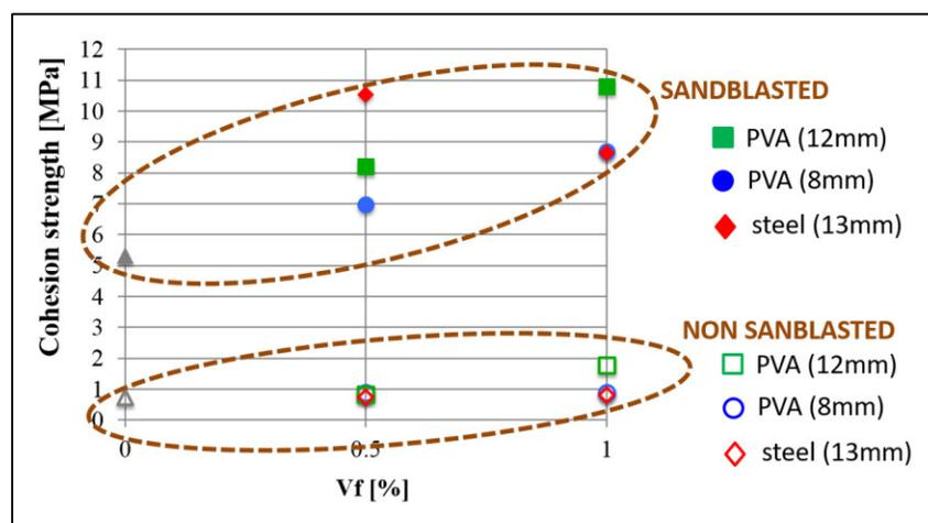
Figure 1: Cohesion strength vs fiber volume fraction ( $V_f$ )<sup>1,2</sup>
